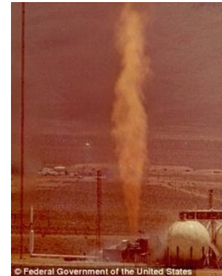
Phoebus-2A (Project Rover) 4000 MW(th) Thrust: 250,000 lbf Isp: 820 s Firing Duration: 32 minutes Test Date: 1968
