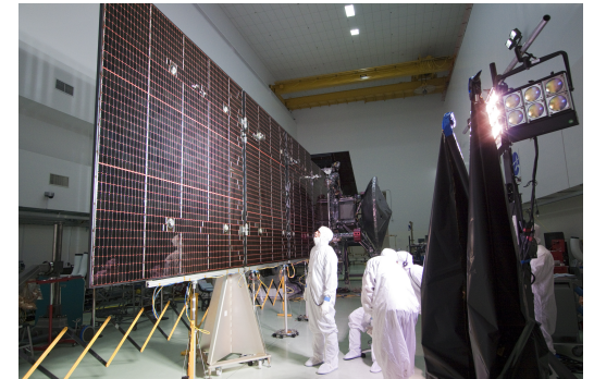
1 of JUNO's 3 Solar Arrays Panel Mission Output: ~150 W
